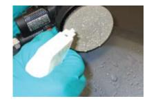
Use 3M<sup>™</sup> Trizact<sup>™</sup> Fine Finishing Abrasive Discs P3000 76mm (50415) over the area to speed up polishing time.
