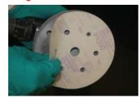
Excess defects are removed by using 3M<sup>™</sup> 260L Fine Finishing Discs P1200/1500 (50239/50238). Use with 3M<sup>™</sup> Hookit<sup>™</sup> Soft Interface Pad (05774).
